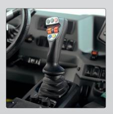
A **joystick** with armrest, which combines the main hydraulic functions, change of direction, change of steering modes, PTO mode and cruise control, allows an ergonomic operation.
